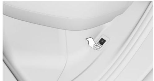
Pull the switch and fold the rear seat backrest forward.
