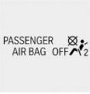
The indicator light is continuously illuminated when the seat is not occupied or when a child is detected on the seat in a provided child restraint system as intended. The airbags on the passenger's side are not activated.
