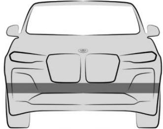
The ultrasonic sensors of the parking assistance systems are located in the area shown.
