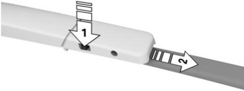
2. Attach a new wiper blade. The wiper blade must engage audibly.
