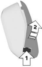
2. Slide out the integrated key at the open side of the vehicle key.
