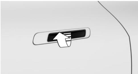
Press and hold the button in the recessed grip to unlock the vehicle and open the rear door.
