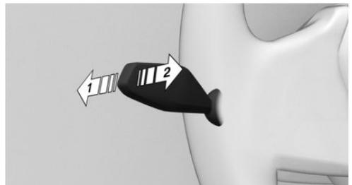
To reactivate the Automatic High Beam Assistant, press the turn signal lever up, arrow 1.
