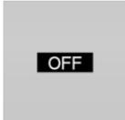
The lettering OFF in the instrument cluster indicates that drive-ready state is switched off and standby state is switched on.
