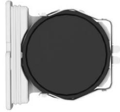
4. Insert a type CR 2032 3V battery with the positive side facing down.
