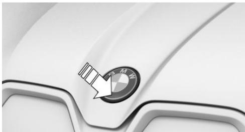
The washer fluid reservoir is located under the hood. Push on the emblem to open the tank. The lid opens when the vehicle is unlocked.
