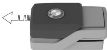
4. Insert the removed cover on the back side of the fragrance cartridge.
