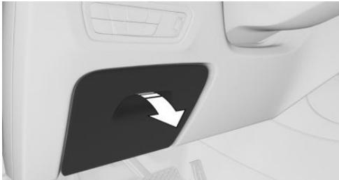
Press the button on the exterior and open the cover, arrow.
