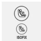
The corresponding symbol shows the mounts for the lower LATCH anchors.
