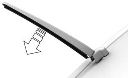
2. Attach a new wiper blade. The wiper blade must engage audibly.
