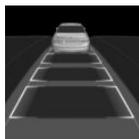
**No distance control display, as the accelerator pedal is being pressed.**
