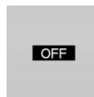
The letters OFF in the tachometer indicate that drive-ready state is switched off and standby state is switched on.
