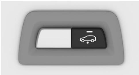
When the tailgate is opened, the vehicle can be lowered to the entry level and raised again by pressing the button. The flashing of the LED in the button indicates the level change.
