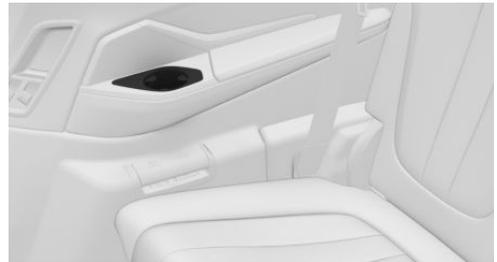
The cup holders are located in the left and right side trim panels in the rear.
