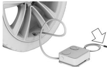
5. With standby state switched on or the engine running, switch on the compressor.
