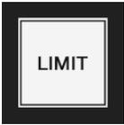
If the detected speed limit has been exceeded, the indicator light will flash.
