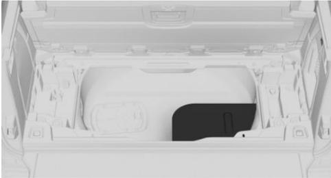
The Mobility System is located in the storage compartment under the cargo floor panel. Fold up the cargo floor panel.
