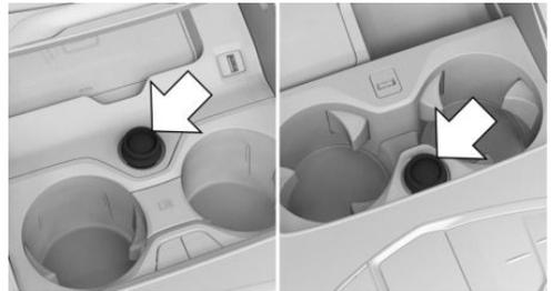
A socket is located between the cup holders in one of the marked positions.
