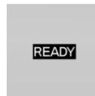
The letters READY in the tachometer indicate that the Auto Start/Stop function is ready to start the engine automatically.
