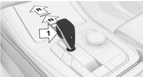
4. Release Start/Stop button and selector lever.
