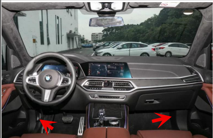
1.1 Disassembly of the interior: remove the interior at the position indicated by the arrow;
