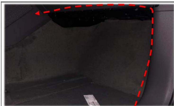
2.7 Left motor wire, positive pole threading:left motor wire is arranged as shown in the figure
