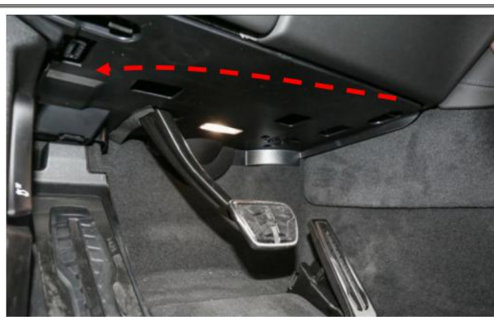
2.8 Left motor cable, positive pole threaded. The left motor line is arranged as shown
