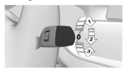
Turn the outer switch upward.
