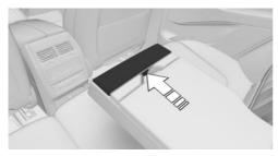
Fold the center armrest forward. Press the button and fold out the cup holder fully.
