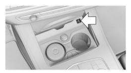
If the vehicle is equipped with thermo-cup holders, a USB interface is located in the center console.
