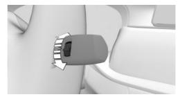
Turn the thumbwheel on the wiper lever.
