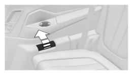
One USB interface each is located in the side trim panel in the rear. Unfold the cover.
