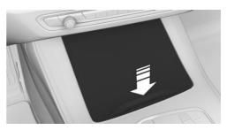
2. The ashtray is located in a cup holder. Fold the ashtray cover upward.
