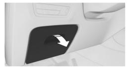
Press the button on the exterior and open the cover, arrow.
