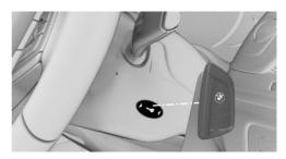
It is not possible to switch on the drive-ready state if the remote control has not been detected.
