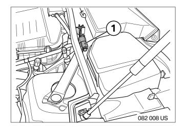
2.1Locate 3-position black hood switch connector(1). Remove securing tape and protective cover.
