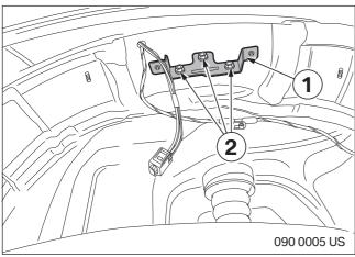
3.4 Install siren bracket (1) over threaded studs and secure in place with three M6 hex nuts (2).
