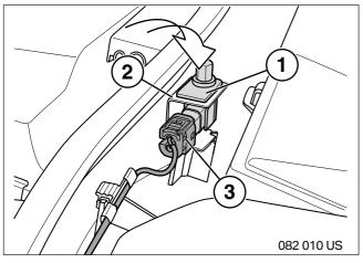
2.3 Insert hood switch (1) into hood switch bracket (2).
