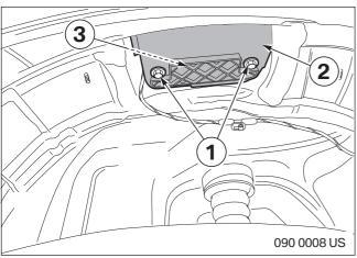
3.8 Use M6x18 hex bolts (1) to secure mounting plate (2) to bracket (3).
