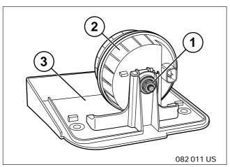
3.5 Position siren (2) to mounting plate (3) and secure in place with M6 hex nut (1).
