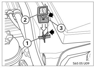
Note: Make sure "corner notch" on bracket faces reward and fits into base mounting tab as shown.
